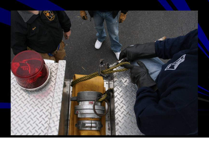
Feed the looped end of the rope through the metal ring. Pull the rope tight, so it captures the hose, wrench and hydrant fitting
