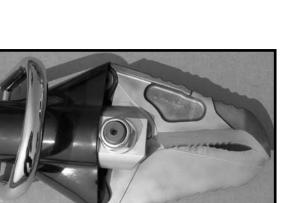
After use, position the blades slightly open for storage. Protect the tool from moisture or store in a moisturefree location. Secure in adequate storage space to prevent damage to the tool and kinking of the hoses.
