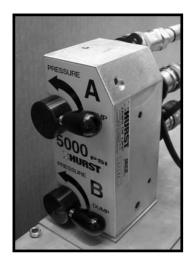
Before connecting the hydraulic hoses, place the power unit by-pass valve in the DUMP position
