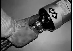
Start the power unit and move the operating lever on the power unit bypass valve to the PRESSURE position. Operate the cutter by turning the control valve to the left to open the blades and to the right to close the blades. If the tool does not operate correctly, make sure the quick disconnects are properly connected (Step 4). If needed, refer to the troubleshooting section of this manual.
